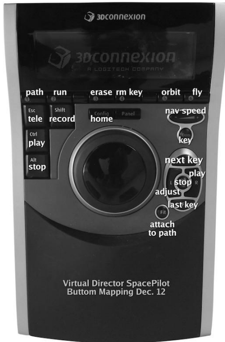
Figure 4: Customized SpacePilot™ button mapping for Virtual Director commands and direct input for a variety of functions including flight through data, recording and editing camera paths through data.
