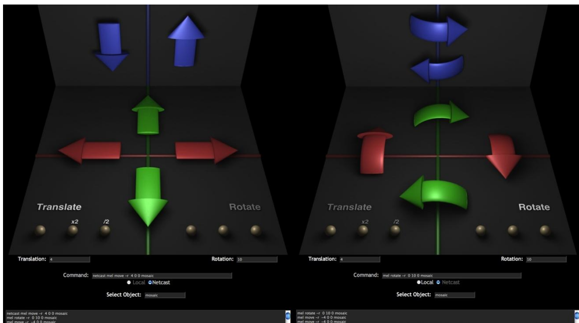
Figure 5: NCSA created and tested a web graphical user interface prototype for nudging selected DCH objects in the stereoscopic virtual scene and for also sending these commands to session collaborators. Figure 6: There are settings for modifying the amount of translation and rotation for each click or touch on a tablet and a history of commands being sent.
